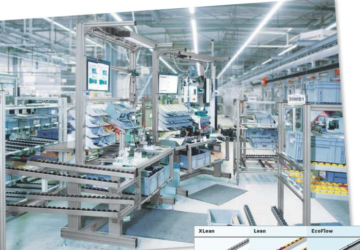
When designing your flow rack system, it is essential to know which materials will be supplied in what quantity and in which containers. The number of parts and containers, their type, their dimensions and their weight all need to be taken into account.
